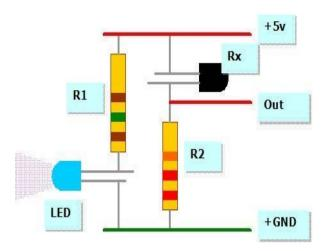
Figure 1: IR Sensor Element
