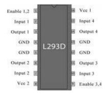
Figure 4: L293D Motor Driver Pin Diagram
